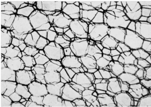
E. Solid foam. A section of expanded polystyrene, showing thin membranes and polyhedral cells. (Sample kindly provided by Mr. A. Cooper, Messrs. Expanded Plastics, Ltd.)
